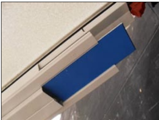
19. Fit supplied infill plate (BLBC001/2) from kit (BLBC001) and fit between L sections at top of hip bolster bar.
