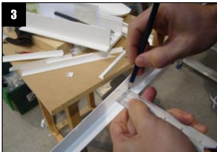
Mark off the angle to size.
