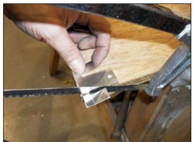
14. Cut BLUC001 as shown. With bent arms pointing upwards, a left hand bracket requires the right hand arm removing and vice versa.
